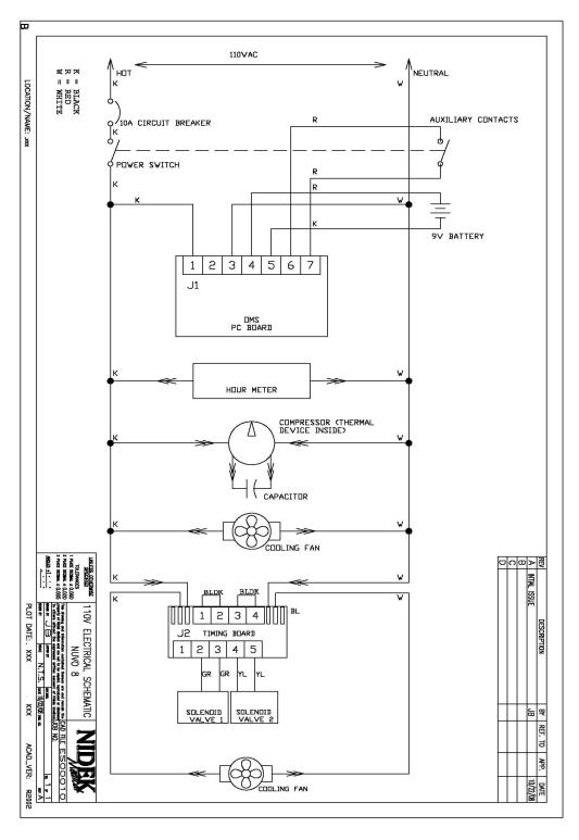
A-3, 115 Volt Electrical Schematic ES00010, with OCSI
