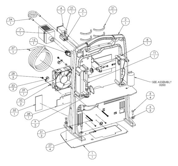
A-5, MAIN STRUCTURE ASSEMBLY FRONT VIEW
