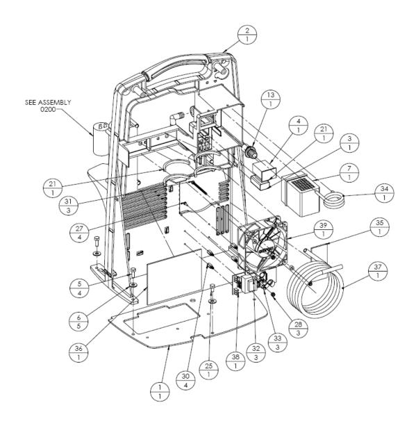
A-5.1, MAIN STRUCTURE ASSEMBLY REAR VIEW
